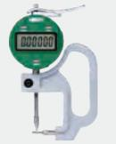
TUBE THICKNESS GAUGES
