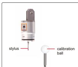
basic probe set (optional), includes .039" DIA, .079" DIA, .118" DIA styli, .984" DIA calibration ball, measuring accuracy is .0004"
