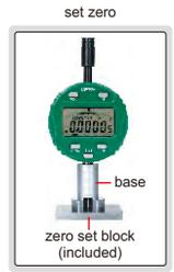
measure peak-to-valley height of blast cleaned surfaces
