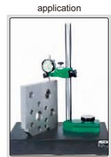
rigid construction, designed to make comparison height measurement (set zero with gauge block then measure height of workpiece) with dial indicators or digital indicators (variation of measuring force is high)
