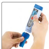
electrodes can be replaced
