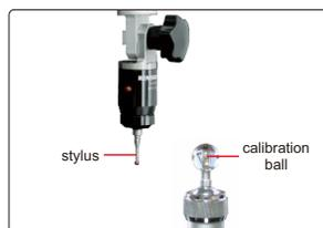
includes .079" DIA/Ø2mm and .118" DIA/Ø3mm styli, .984" DIA/Ø25mm calibration ball, measuring accuracy is .0004"
